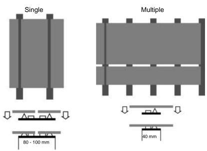
Required width of substructure battens for the use of the SikaTack -Panel System. The full height of the façade panel must be bonded.
